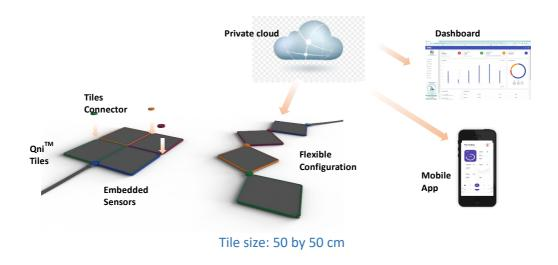
Takaro's tiles are equipped with high sample-rate multi-touch and proximity sensors, together with directional sensors for tile configuration detection and smart adjustment to exergame activities.
